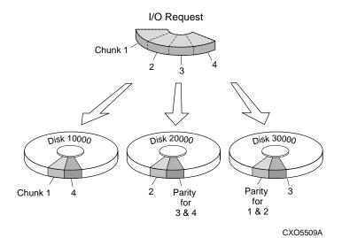
Figure 3–7. Parity Ensures Availability; Striping Provides Good Read Performance
